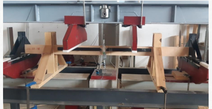
Figure 11. Bending test on structural sized specimens.
