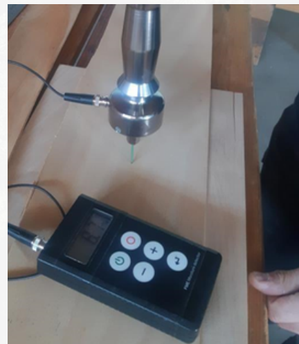
Figure 6. Moisture control of sheets with xylohygrometer.
