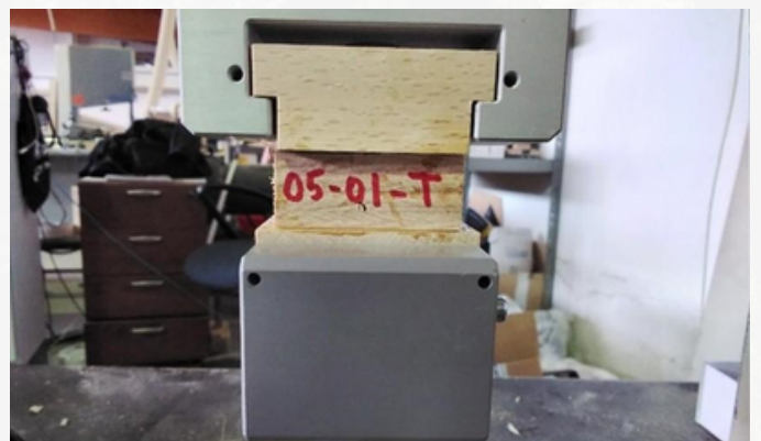
Figure 13. Perpendicular tensile test on fiber.
