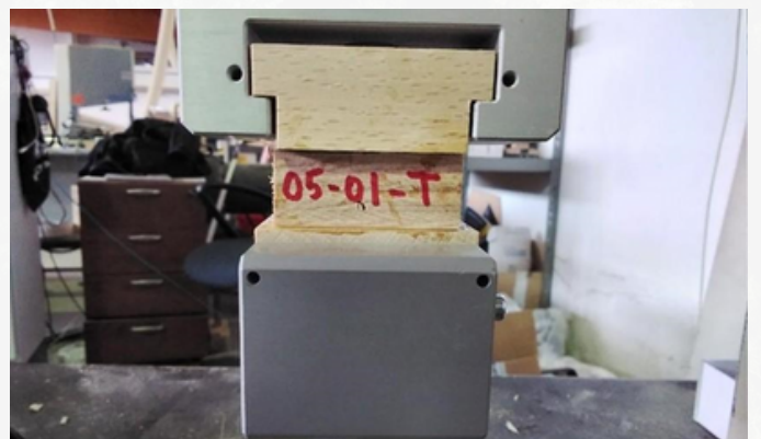
Figure 13. Perpendicular tensile test on fiber.
