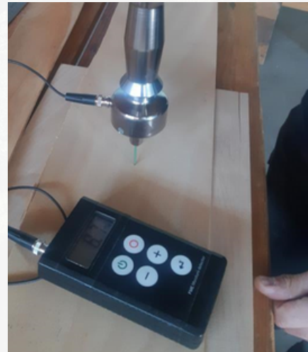
Figure 6. Moisture control of sheets with xylohygrometer.
