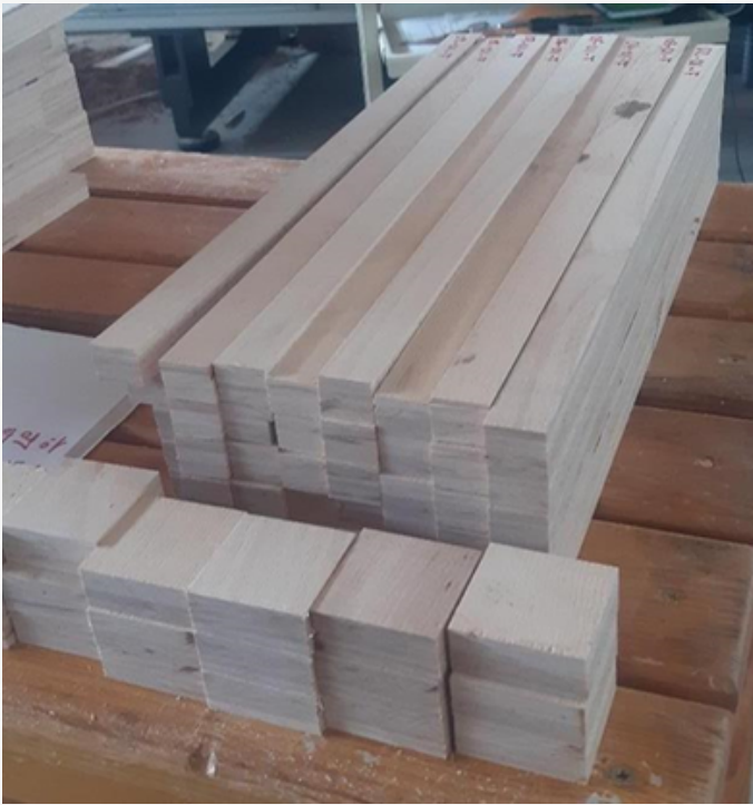
Figure 10. Small specimens for bending tests (upper) and for tensile tests perpendicular to the fiber (lower).
