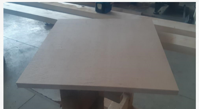
Figure 9. 500x500 mm panel, used to produce small specimens.
