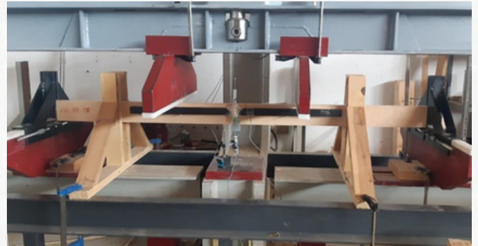
Figure 11. Bending test on structural sized specimens.
