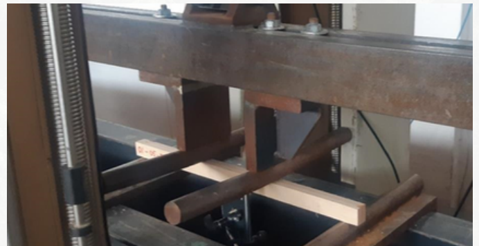
Figure 12. Bending test on small dimension specimens.
