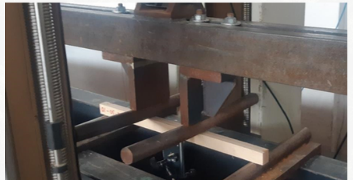
Figure 12. Bending test on small dimension specimens.
