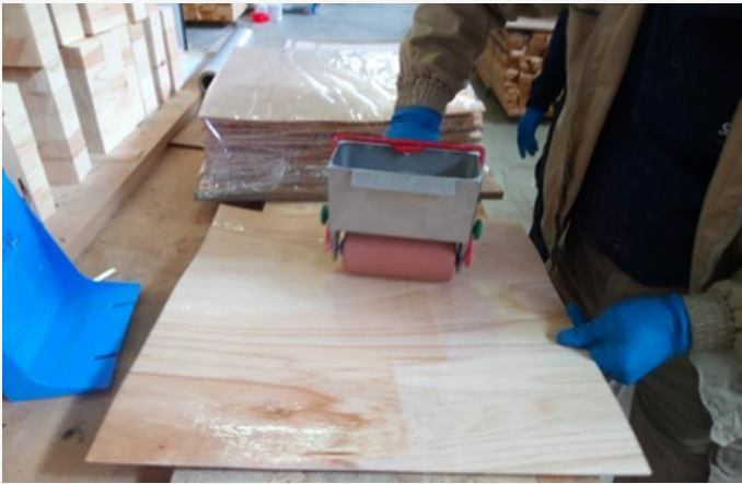
Figure 7. Gluing and placement of veneers.
