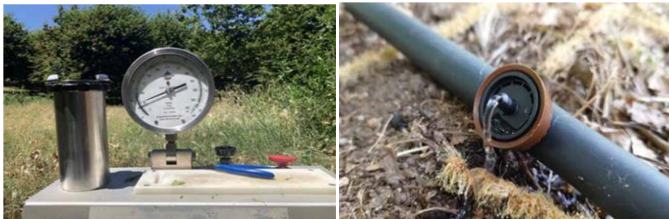
Figure 1: Pressure chamber for measuring the water potential of the trunk (on left) and drip irrigation (on right).
