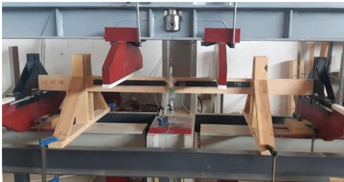
Bending test on structural sized specimens
