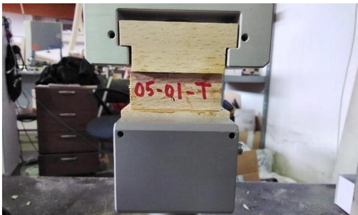
Perpendicular tensile test on fiber
